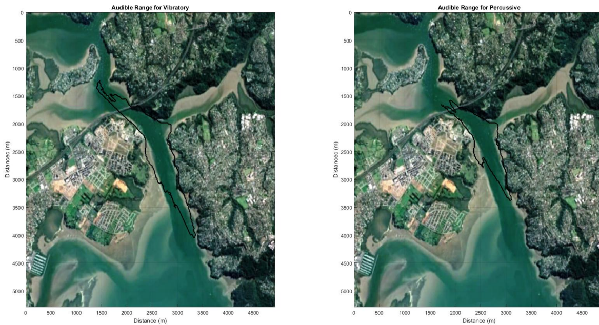
Figure B.6: Plot showing the limits of audibility for common dolphins during the vibratory (left panel) and percussive (right panel) piling.
