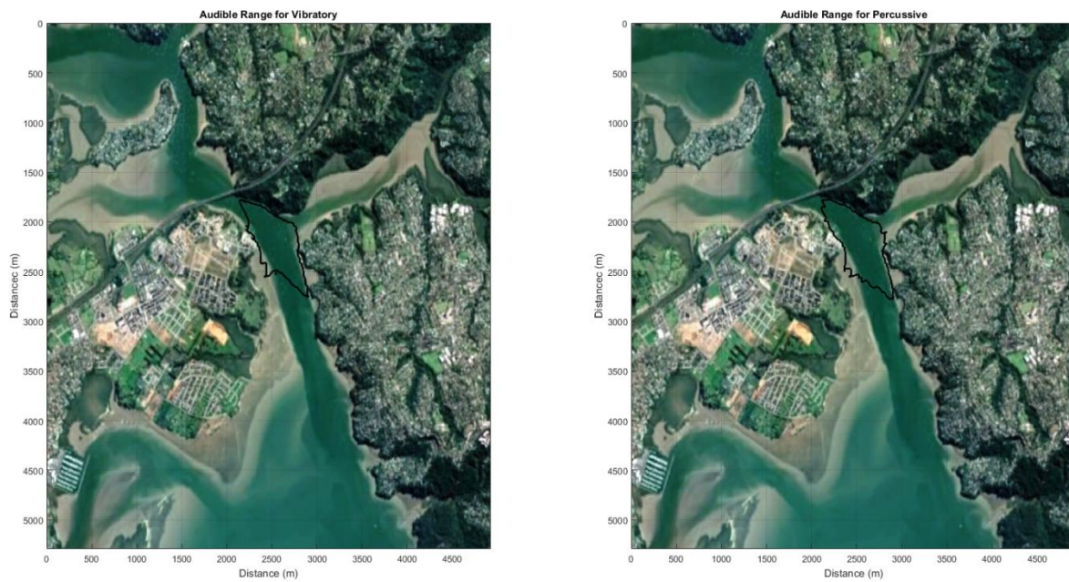
Figure B.7: Plot showing the limits of audibility for fish during the vibratory (left panel) and percussive (right) piling.
